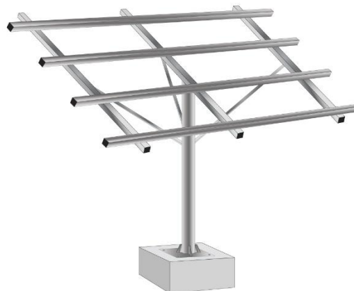
(e) MMS for solar water pumping system
