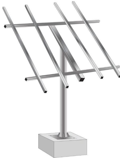
Fig.1.10: Placing Solar rack
